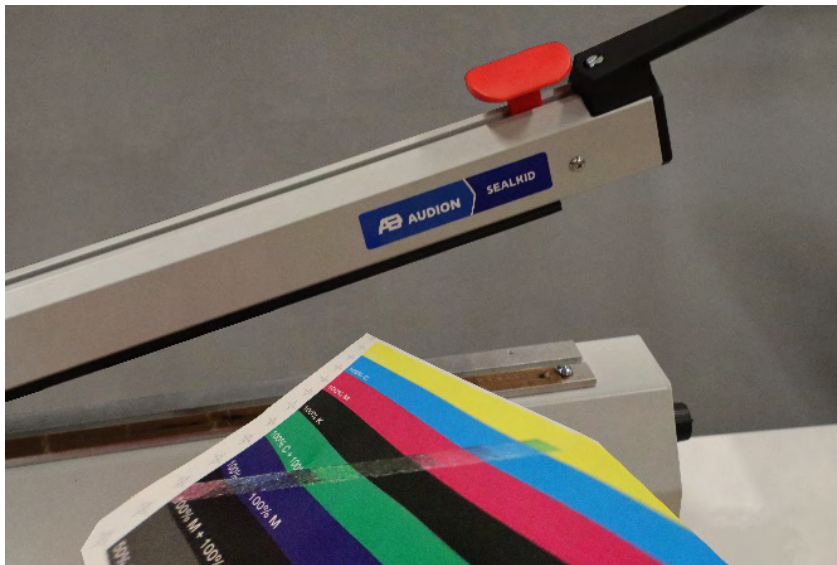
Conventional dry toner layers have insufficient seal resistance for use in flexible packaging, in contrast to TITON dry toner. (Source: pack.consult)
