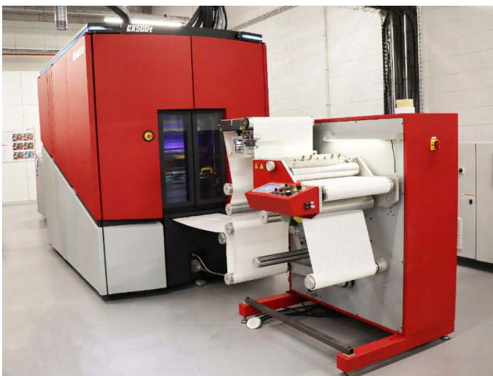
The Xeikon CX500t has an LED curing unit for crosslinking the TITON toner. (Source: pack.consult)
